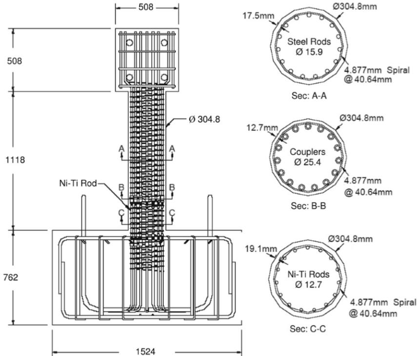
Figure 1. Details of SMA-RC column (Saiidi and Wang, 2006)
