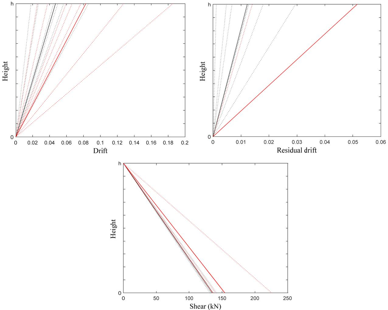
Figure 3. Maximum drift, residual drift and maximum shear of the column subjected to each ground motion (dotted line) and the mean of the responses of the 7 cases (solid line), (Fling step containing: red lines, Far-fault: black lines)
