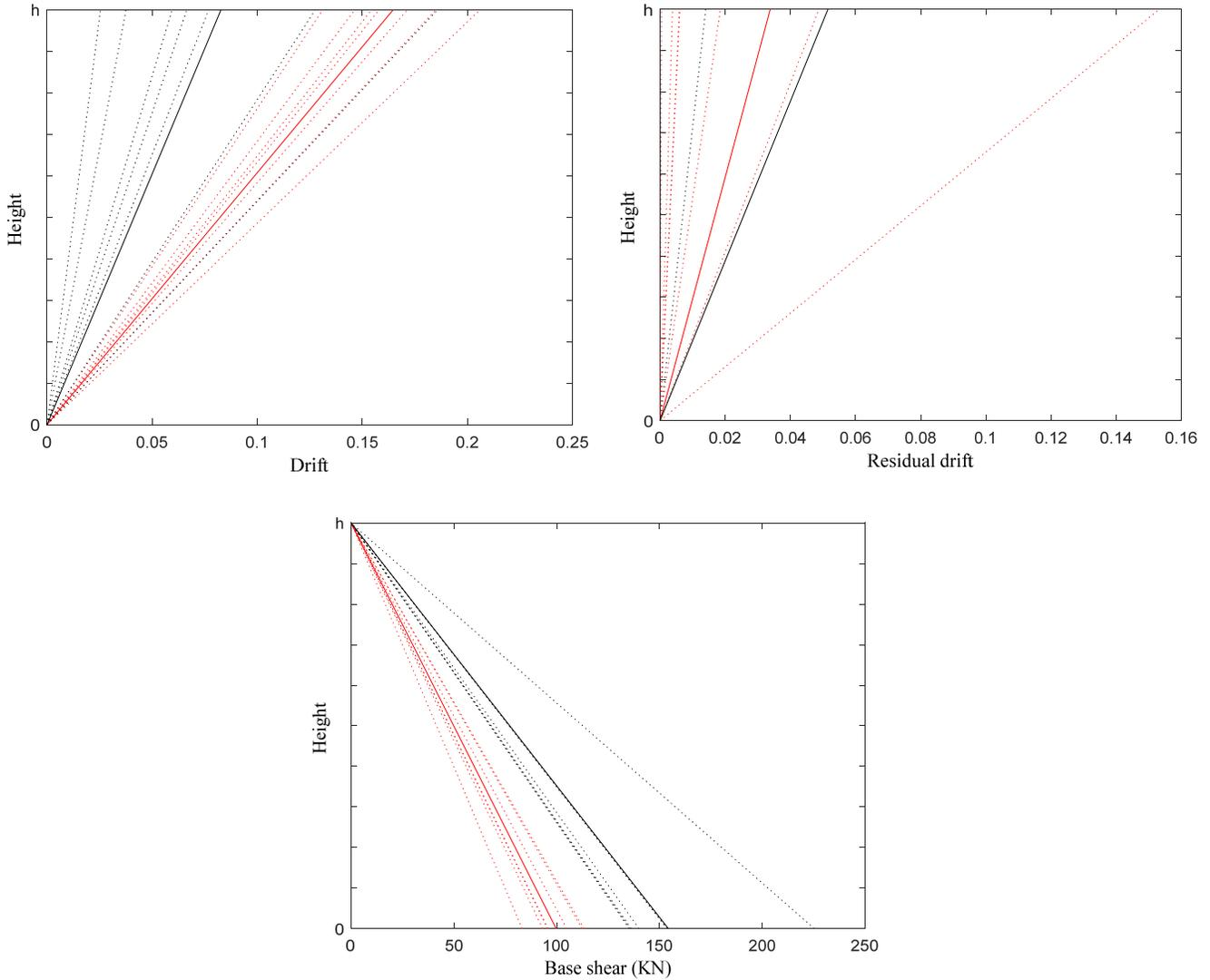
Figure 5. Maximum drift, residual drift and maximum shear of the column subjected to each ground motion (dotted line) and the mean of the responses of the 7 cases (solid line), (SMA: red lines, No SMA: black lines)
